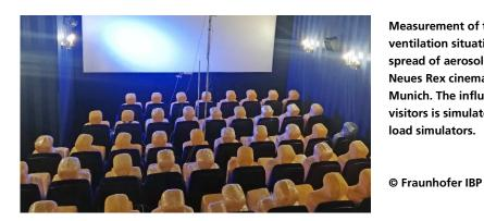
Measurement of the ventilation situation and spread of aerosols in the Neues Rex cinema in Munich. The influence of visitors is simulated by heat load simulators.
